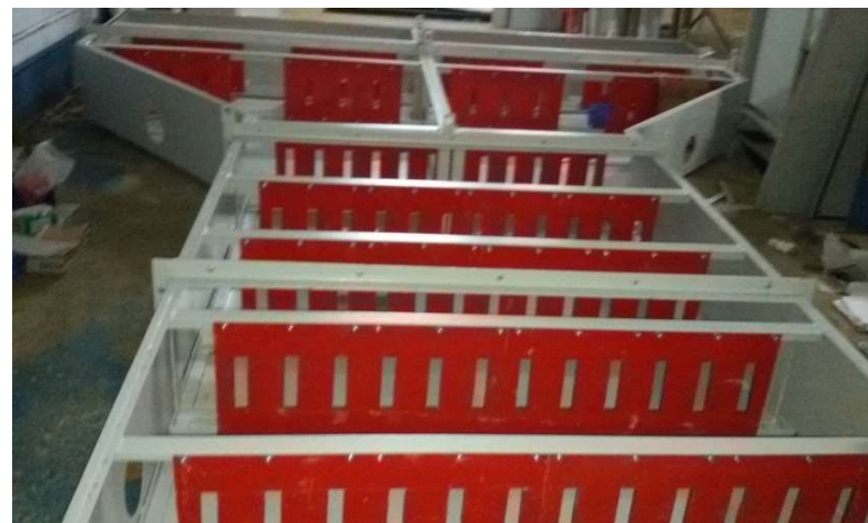
5000A Bus duct
