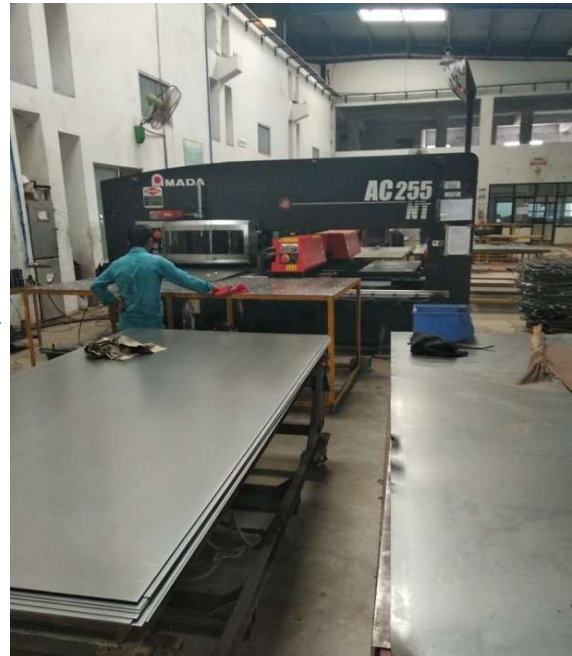
Punching process on Amada AC 255 NT
